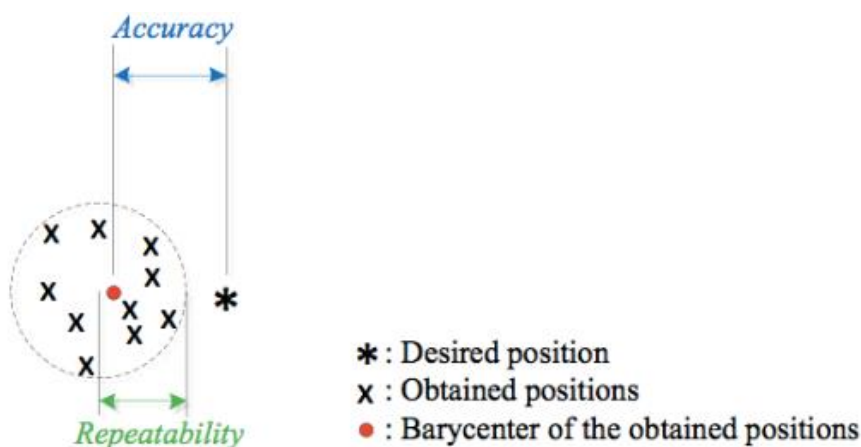
Fig.1. 2D illustration of the geometric meaning of repeatability accuracy
