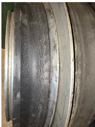
Fig. 2. Ski lift rubber seal wear
