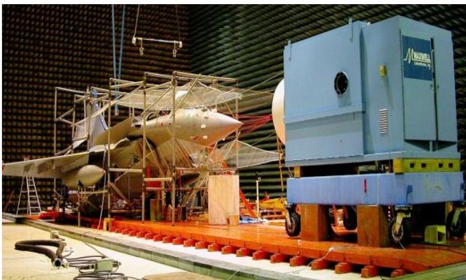
Figure 8 –Lightning indirect effects tests
