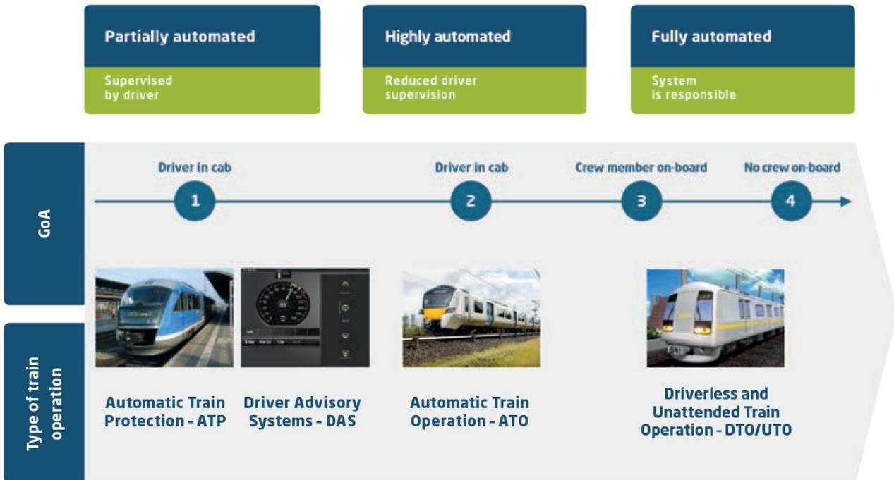
Fig. 1 Grades of Automation and Train Control Systems [3]
