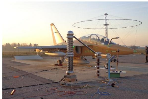
Figure 9 The M-346 aircraft during ESD testing
