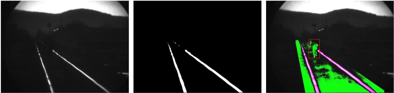
Fig 4. Object between rail tracks – marked as an obstacle [7]
