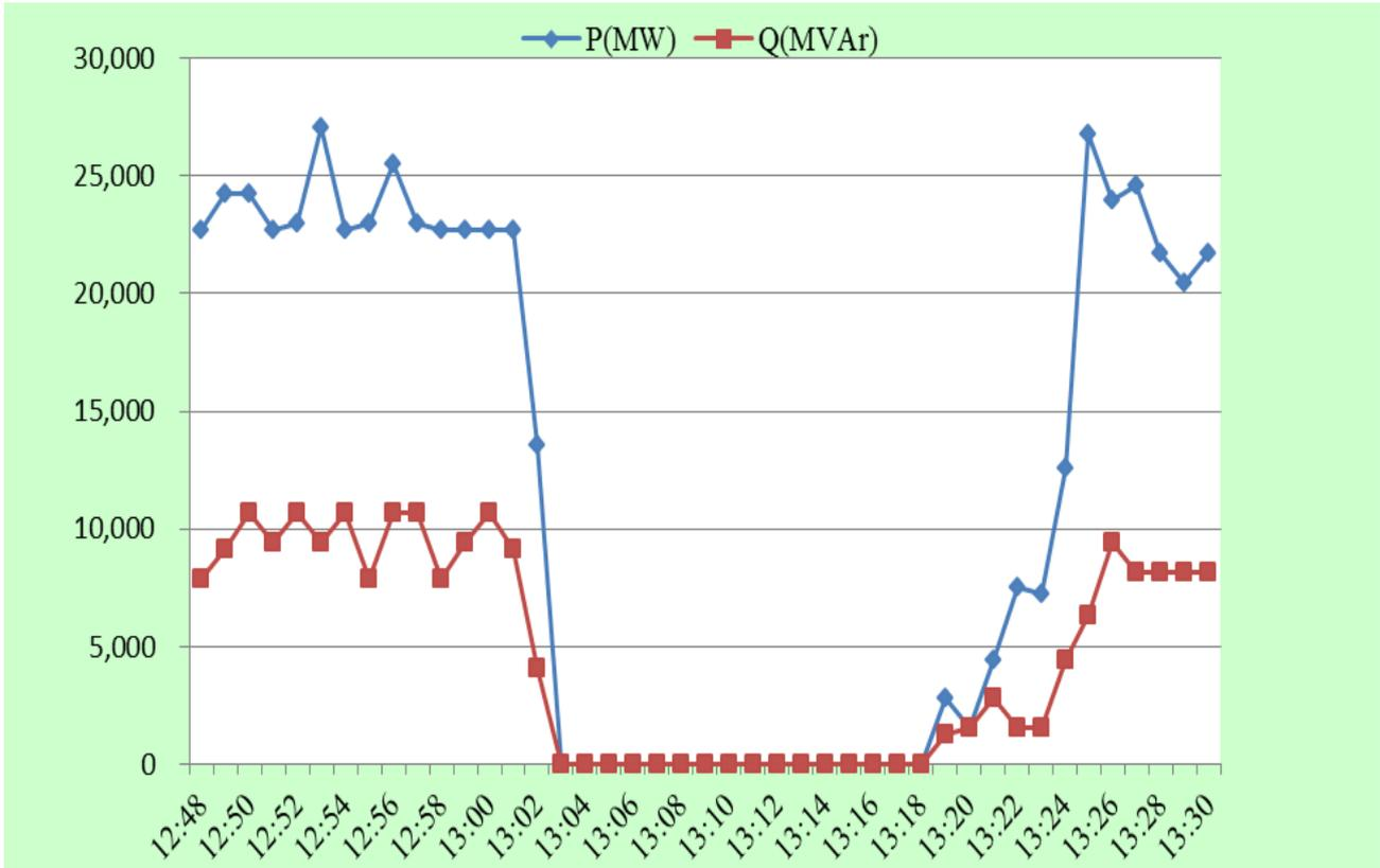
Fig.5 The P and Q during fault 08/09/18
